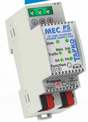
MECps640 Line-/Area Coupler with integrated 640mA KNX power supply
