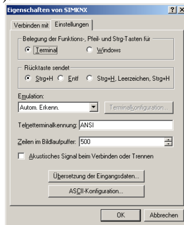
Figure 27: using SIM-KNX with Microsoft hyperterminal: where to find ASCII configuration
